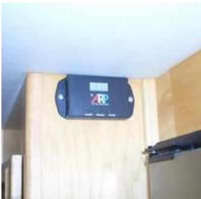
Why do RV refrigerators overheat and how does ARPRV help? There are a variety of reasons that can occur in normal operation. One of the best known is off-level operation, which interferes with the gravity flow of refrigerant back to the boiler and stops the cycle while the heater (LP gas or electric) continues to raise the boiler temperature.
