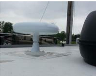
As you can see, the finished product is lower than the air conditioner shroud- and may not be suitable for those RV's with the aluminum side trim higher than the top of the motor home.
